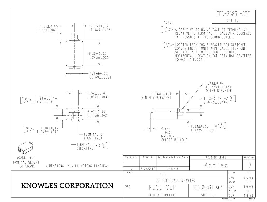
THE FED-26831-A67 IS A FERROFLUID AND TYPE III DAMPED ED RECEIVER WITH A PEAK OF 4dB RELATIVE TO THE SENSITIVITY AT IKHZ UNDER CONSTANT VOLTAGE DRIVE CONDITIONS. THIS MODEL HAS INCREASED DCR/IMPEDANCE RATIO.
